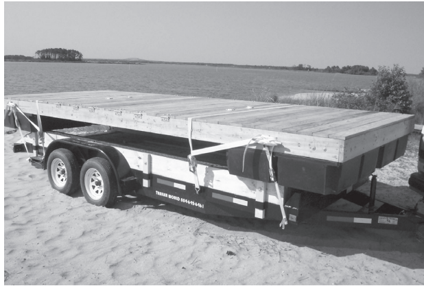
Floating upweller on trailer, ready to launch into water
